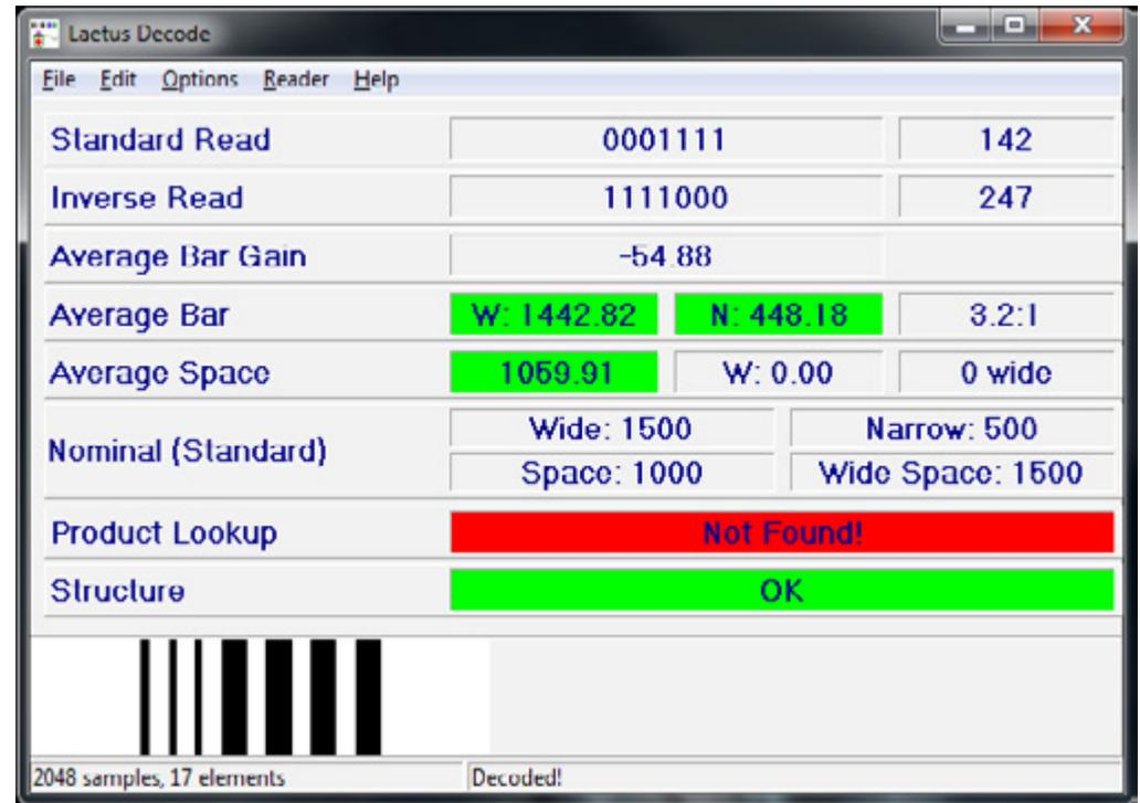
The **Laetus Decode** window provides the binary pattern data followed by the value of the data, and shows this in both directions. All the measurements are expressed in  $\mu\text{m}$  (thousandths of a millimetre), and the entries are coloured green or red depending on whether they are in specification. An image of the symbol that has been read is also shown in the window.
